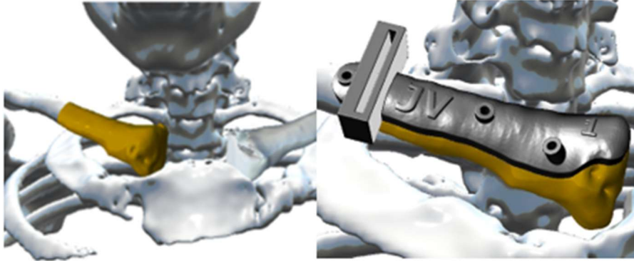
Figure 25: Virtual models. The virtual model of the anatomical defect (Left, yellow area). The virtual model of the custom cutting guide (Right, holes for fasteners and cutting slot shown).
